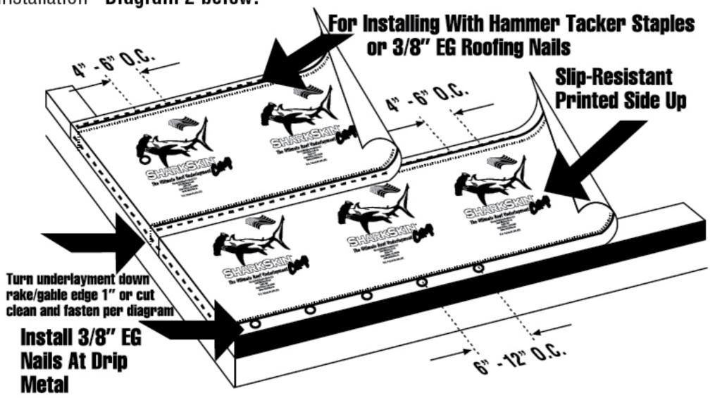
The underlayment shall be fastened as necessary to hold in place to allow for safe walk ability for the installer. \*HAMMERTACKER STAPLE INSTALLATION. COPYRIGHT ©2009 by Kirsch Research and Development LLC.
